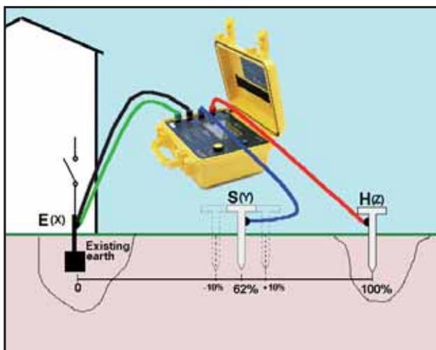
The positioning of the two auxiliary electrodes in relation to the earth connection to be tested E(X), is crucial. For correct measurements, the "auxiliary connection" providing the reference potential (S) must not be positioned in the areas influenced by earths E & H due to the flow of the current (i).
