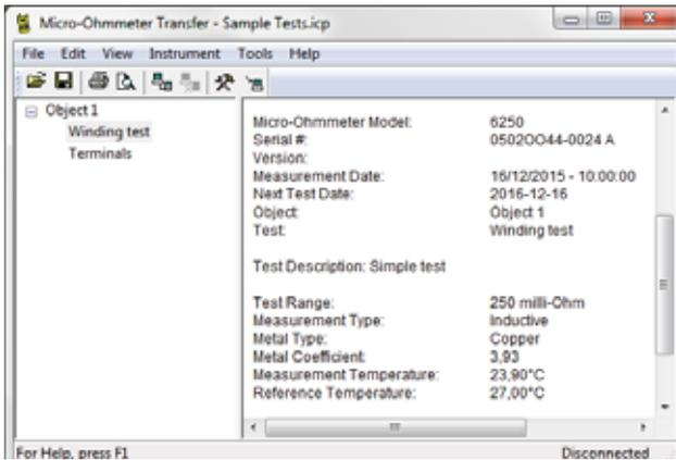
MOT MODULE Results of motor winding test
