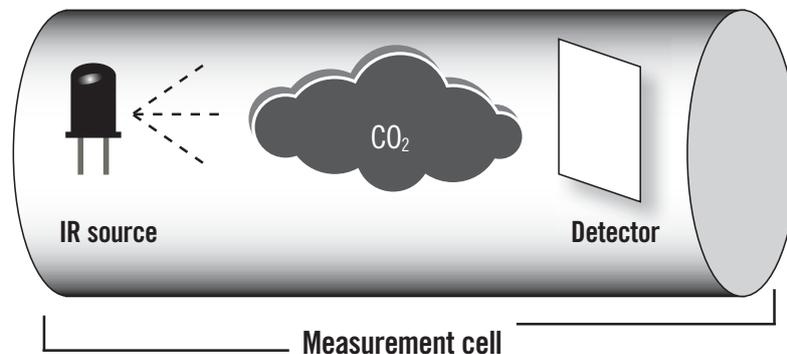
CO<sub>2</sub> and other gases absorb IR radiation in a “specific” way.
