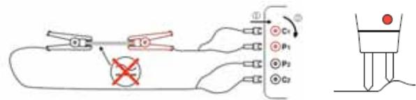
**The micro-ohmmeters must offer a resolution of 1  $\mu\Omega$  or even 0.1  $\mu\Omega$ , a wide measurement range and compensation of the thermocouple effects by inversion of the measurement current.** To ensure operator safety, the equipment must be protected against accidental overvoltages, prevent measurement in the presence of a disturbance voltage and trigger automatic discharging after measurements on inductive objects.
