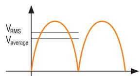
For a sinusoidal AC voltage
