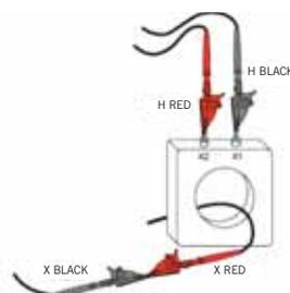
excitation current can identify problems in the magnetic core of the transformer, such as type and thickness of the material, mechanical stresses and air-gap and assembly variations.
