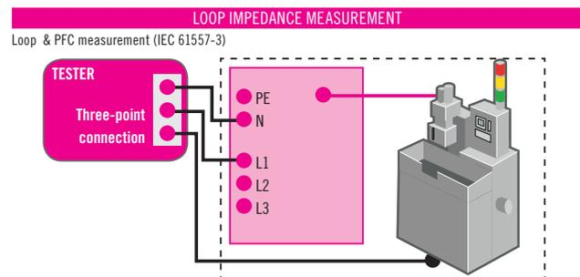
By measuring the loop impedance and calculating the prospective fault current (PFC), you can check that the automatic cut-off systems or fuses are appropriately sized.
