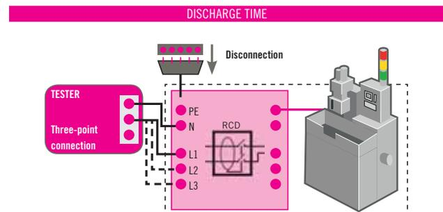
When the machines are disconnected, high-value capacitors may supply a hazardous voltage. This test measures whether the time taken by the discharge voltage to reach a non-hazardous value complies with the requirements ( $< 5s / < 1s$ ).
