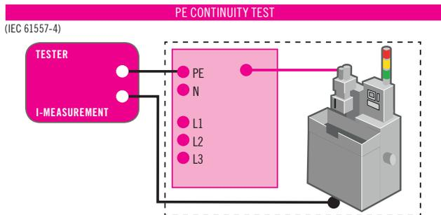
Used to check whether the resistance measured corresponds to the cross-section and length of the PE conductor.
