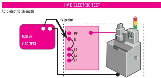
The AC dielectric test can be used to confirm the device's ability to function at its operating voltage. These tests are performed at a higher voltage than the normal operating voltage.
