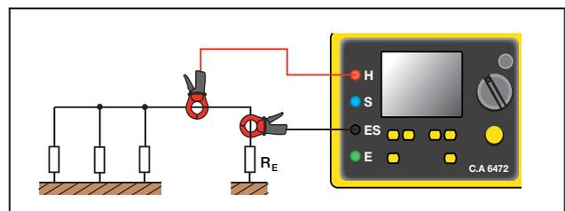
It is also possible to use the 4-pole + clamp method, which requires auxiliary stakes but allows precise measurement of the earth resistance.
