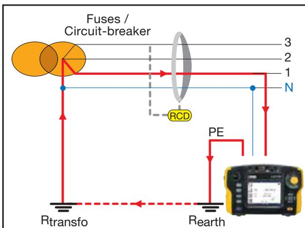
**Note:** on TN or IT (impedant) systems, the loop impedance measurement can be used to calculate the short-circuit current and thus to size the protective devices correctly.
