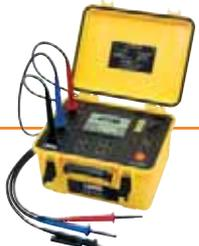
**6** 15 kV insulation testing
