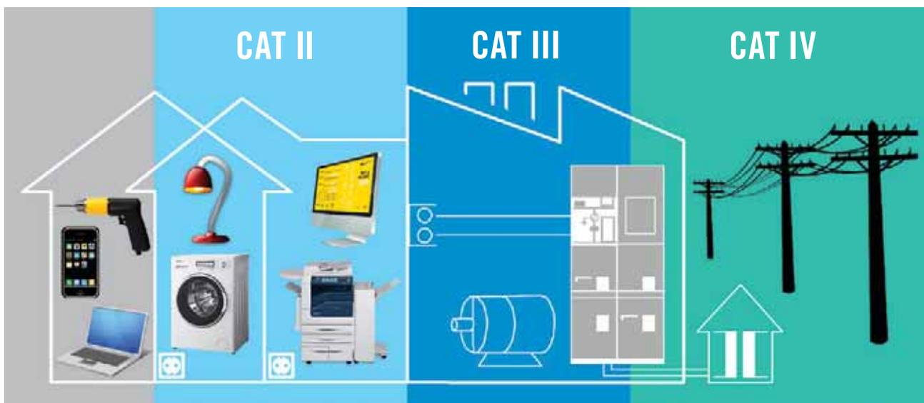
**CAT II : Measurements on circuits connected directly to the low-voltage installation.**
