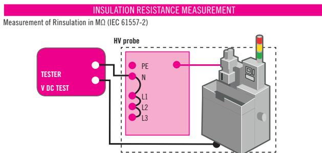
By measuring the insulation resistance, it is possible to detect faults due to deterioration or pollution and mould.
