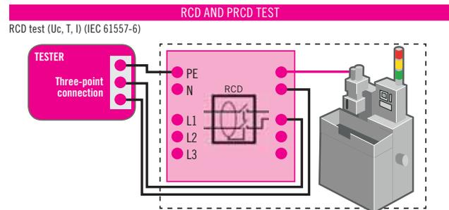
The RCD test can be used to check operation of the RCDs.
